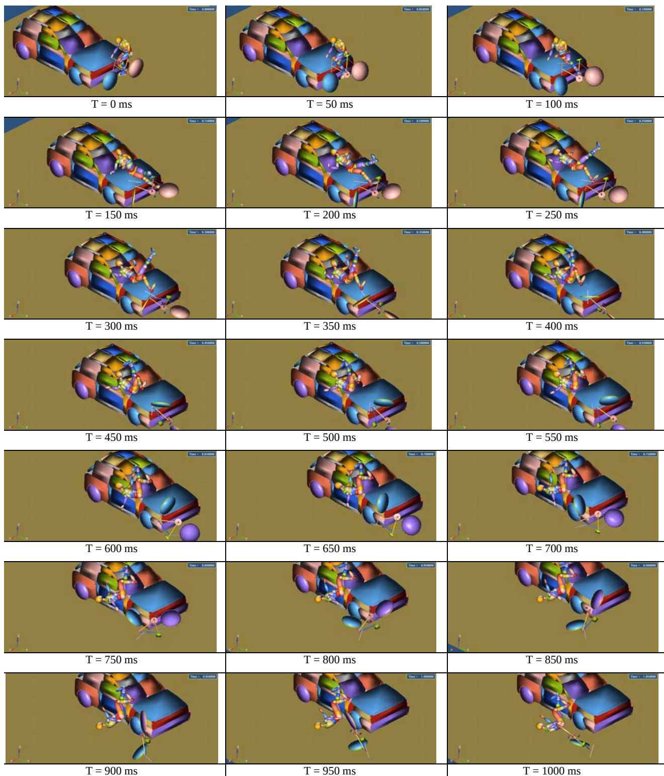
Figure 6 Motion of bicycle rider in front-to-side-side crash (Car velocity = 25 km/hr, Point of impact at car centre)
